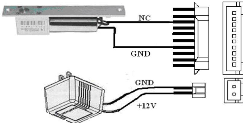
2、 NO lock connection ( Access control Station and lock powered by one adapter together , Jump 2.3 pin closed ) .
