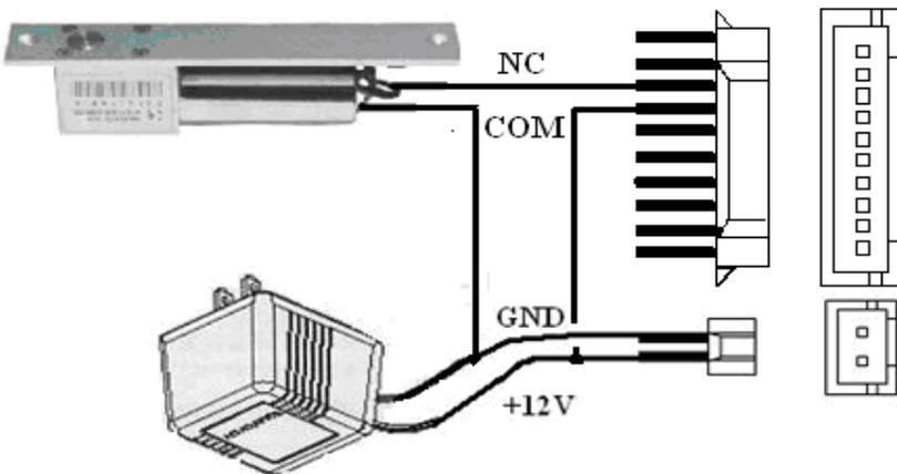
4. the output relay signal by Access control station, NO lock connection ( Access Control station and lock powered by independent adapter
