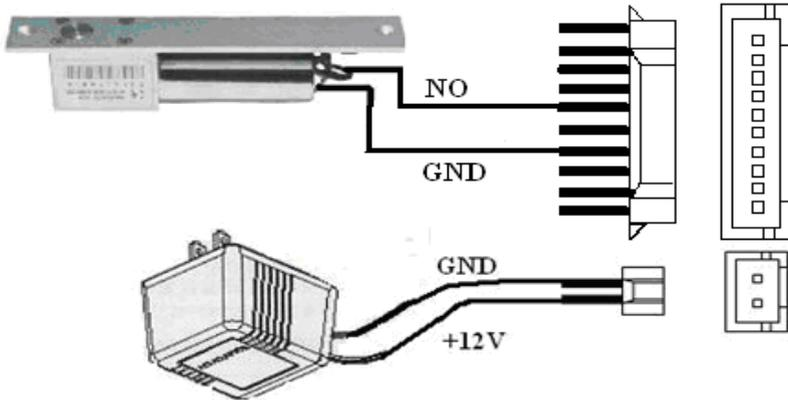
3. the output relay signal by Access control station, NC lock connection ( Access Control Station and lock powered by independent adapters jump 1,2 closed)
