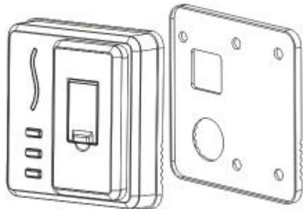
1) Post the moulding board on the wall. Drill holes according to marks on the moulding. (There should be screw holes and lead wire hole)
