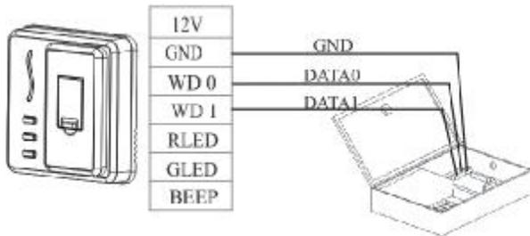
**Note:** 1) The recommended distance between device and access controller should not be more than 90 meters (If a longer distance or an environment with interference, please use the Wiegand signal extender).
