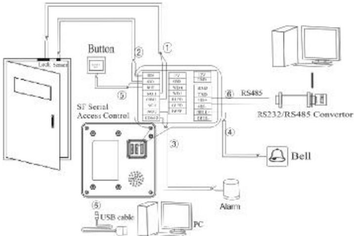
1. When a person has passed the status authentication on the access control device, the device will output the lock control signal to unlock.
