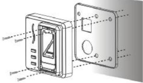
4) Use screws to fix the device and waterproof glue on the wall.
