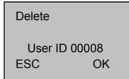
5) The device display the smallest user ID automatically, if you need to modify it, input the desired ID through the keyboard. Press **OK** to confirm and enter the next step.
